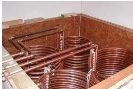
Water and liquid heat exchanger
