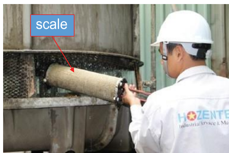
Scale deposited on the device after one month
