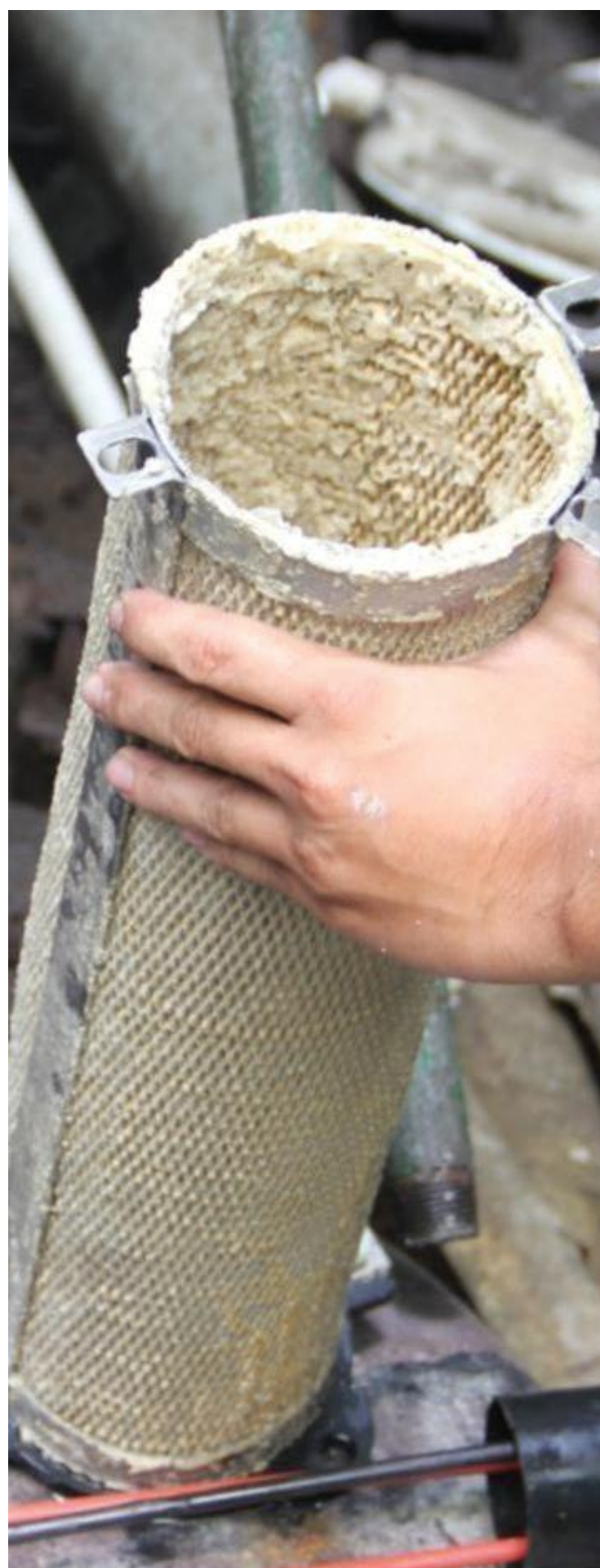
Scale deposited on the device after one month
